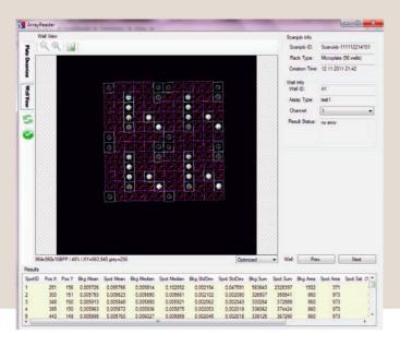
Screenshot of ArrayReader software result window. The captured image was analyzed with automated spot finding algorithms. Result data like spot mean intensity and background mean intensity are listed below the image together with additional statistical data for spot and image qualification.
