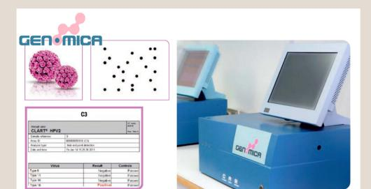
Courtesy of GENOMICA S.A. Unipersonal: The Clinical Array Reader CAR® is used to analyze the multiplexed CLART® HPV2 assay. This colorimetric, microarray-in-well
