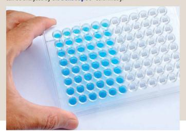
**SensoSpot®** Colorimetry and **SensoSpot®** Fluorescence allow for read out and analysis of planar, low density microarrays in 96-well plates, on microscopy slides or other formats.
