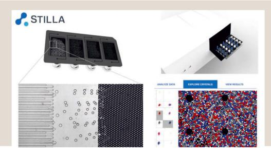
Courtesy of Stilla Technologies: The Naica platform implements Crystal Digital PCR for fast and reliable high-resolution genetic analysis. Sapphire Chips are used to produce droplet crystals by applying surface tension gradients. The fluorescence read out in three channels is realized by the customized Microarray Analyzer and diagnostic results are delivered by an application-tailored analysis software.
