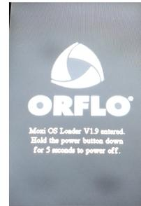
Plug the system into your computer. The system should appear as an external drive (same as a flash drive). The firmware files can then be cut-and-paste or drag-and-dropped to that drive. Following copying of the files, safe eject the system from the computer and touch "OK" on the Moxi Z screen to start the firmware load. The system will shut off automatically when completed.
