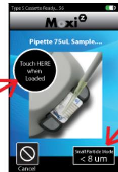
4. Pipette a 75  $\mu\text{L}$  sample into the fill port of the cassette (either test 1 or test 2, depending on which end of the cassette was inserted into the instrument).
