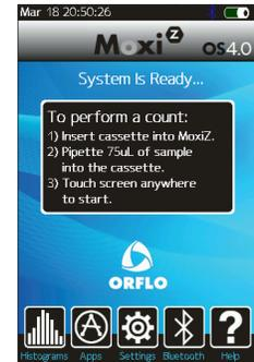
3. Press the tray down and insert a Cassette into the Moxi Z. The **Pipette 75 $\mu\text{L}$  Sample...** screen will be displayed.
