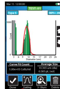
5. For counting most mammalian cells, touch the screen anywhere to start. For counting very small particles (< 8  $\mu\text{m}$  in diameter), the Moxi Z can be run in **Small Particle Mode (SPM)**. In this mode, Moxi Z sets the diameter scale to 2 to 10  $\mu\text{m}$  as the default and performs the count using optimized parameters for the detection of small cells. Press the **Small Particle Mode < 8  $\mu\text{m}$**  button to initiate the test and run in this mode.
