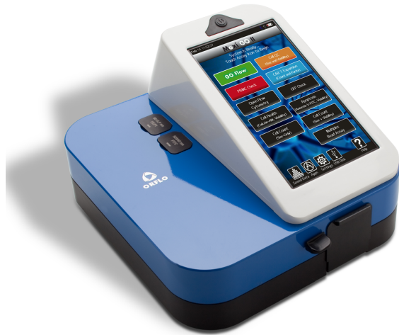
Figure 1 – Orflo's Moxi GO II – Next Generation Flow Cytometer. The Moxi GO II is a configurable flow cytometer with a 488nm laser and up to two fluorescence recording channels (2 PMT's with emission filters at 525/45nm filter and 561nm/LP, respectively).
