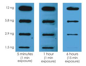
**WesternBright ECL produces a long-lasting signal.** A blot detected with WesternBright ECL can be imaged six hours after substrate incubation. There is no need to rush to the darkroom to image a blot.
