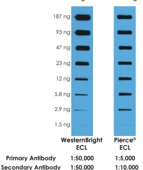
WesternBright ECL detects equal amounts of protein with up to ten times less antibody. Duplicate slot blots containing serial dilutions of transferrin were probed with the antibody dilutions shown, and detected with either WesternBright ECL or Pierce ECL (Thermo Scientific) according to the manufacturers' instructions. The blots were imaged simultaneously on the same piece of film. WesternBright ECL produced the same sensitivity with ten times less primary and five times less secondary antibody.
